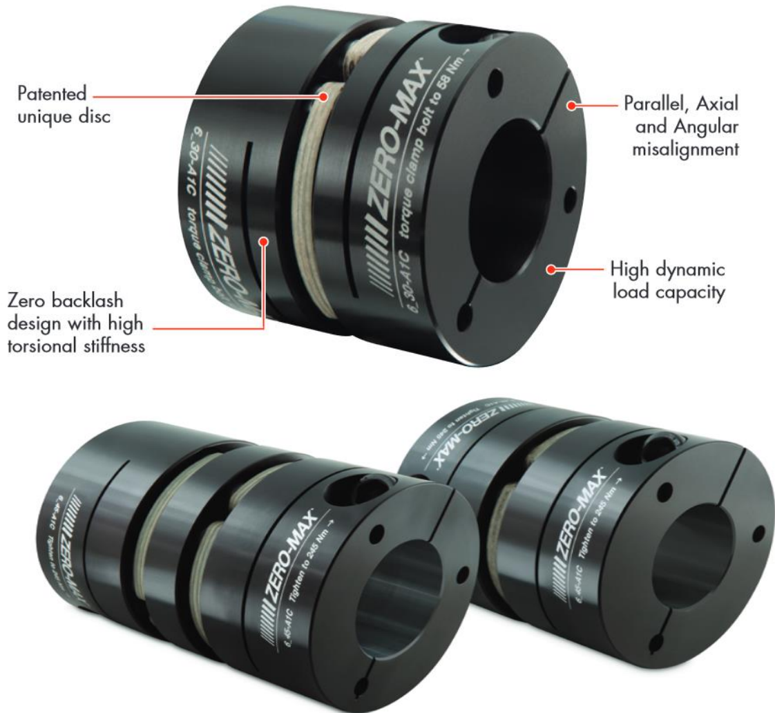
Fig. 5. Double-flex disc coupling
